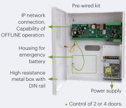
Control of 2 or 4 doors. Up to 4 or 8 entry/exit readers. Wiegand/RS-485 connection.
