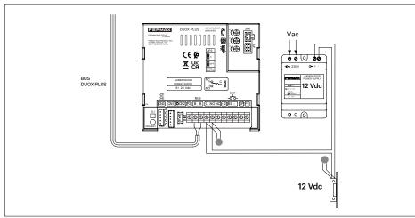
DC ELECTRIC LOCK RELEASE CONNECTION (Consumption < 250 mA) Lock release ref. 29588 is recommended.
