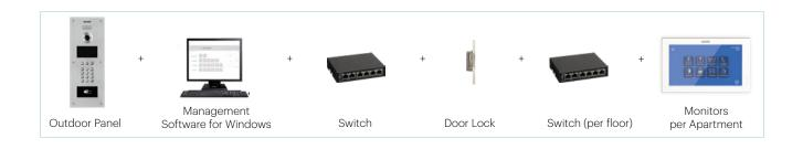
**FERMAX MEET** system is a **100% IP technology based on a Point-to-Point infrastructure**, highly efficient, flexible and powerful.
